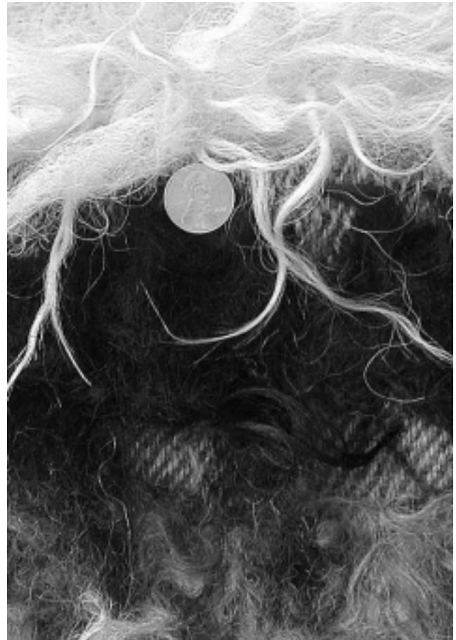
Figure 3. Finished samples: white on white, black and moorit on shades of natural brown (from top to bottom). Overly felted black sample reveals sections of ground weave.
